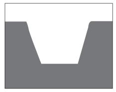
Determine installation location according to lighting plan. Dig hole a minimum of 36" deep and 14" wide. Suitable enough to provide clearance of anchor rod, and proper anchorage for pole.
