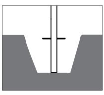
Place pole over installed conduit. Pull branch circuit wiring through pole and out the top.
