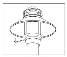
Slide fixture over pole top. Secure with four (4) 1/4-20 screws using a 1/8" allen wrench. Make sure the fixture is completely seated. Do not overtighten.
