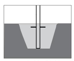
For concrete installation: Fill the hole around the base of pole 24" below grade with clean fill dirt and tamp carefully to prevent further settling. Pour concrete and finish as required flush with finished grade.
