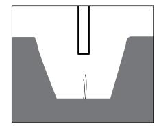
Pull branch circuit wiring through conduit necessary for installation.
