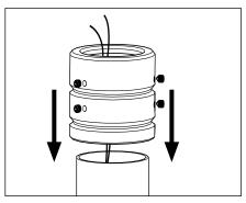
Install tenon adapter provided onto pole top. Tighten six (6) ¼-20" set screws using a 1/8" allen wrench until tenon is secured.
