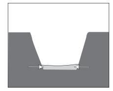
Per DIG-IT Guide, backfill the bottom of pole and bottom of hole with sand for drainage.
