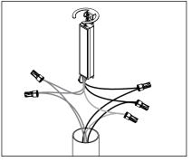
Pull primary branch circuit wiring up to driver bracket location at top of pole. Pull incoming dimming controls to top of pole. Feed through strain relief.
