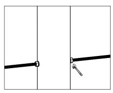
Install provided Anchor Rod into pole through hole. Using and adjustable crescent wrench tighten provided hex nuts against pole base.
