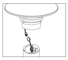
Make secondary connections via quick disconnect from driver secondary side to fixture secondary side.
