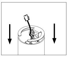
Place connections and driver on bracket into pole. Rest bracket on pole top or tenon.
