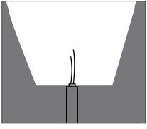
Pole may be directly stubbed into through footing with conduit. Install conduit for branch circuit wiring centered with pole position.
