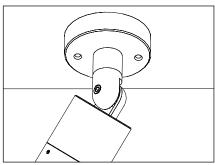
$\underline{\hat{\Lambda}}$  Do not install facing upwards in outdoor installation.
