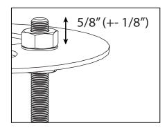
Adjusted anchor rods to project no more than 5/8" with a variance of + or - 1/8" above the anchor plate after installation. The two (2) 1/4-20 nuts on top of the plate may be left in place while concrete is poured.
