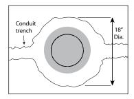
Excavate a hole to the necessary dimensions for fixture placement and conduit runs.
