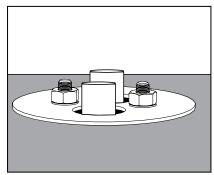
The fixture may be installed by removing the two (2) 1/4-20 nuts and re-using them with a 7/16" wrench to secure the fixture mounting base assembly. See fixture installation sheet(s) for additional information.
