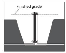
Run conduit inside of the anchor plate center holes prior to pouring concrete. Conduit installation through bottom plate is optional.
