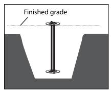
2. Install anchor plate and bolt assembly flush and level with the finished grade.
