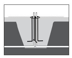
With the conduits in place and the anchor plate properly positioned, secured and leveled, concrete may be poured.
