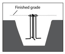
Install anchor plate and bolt assembly flush with the finished grade.
