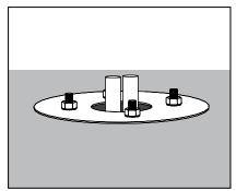
The fixture may be installed by removing the four (4) 1/4-20 nuts and re-using them with a 7/16" wrench to secure the fixture mounting base assembly. See fixture installation sheet(s) for additional information.
