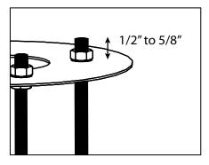
Adjusted anchor bolts to project at least 1/2" but no more than 5/8" above the anchor plate after installation. The four (4) 1/4-20 nuts on top of the plate may be left in place while concrete is
