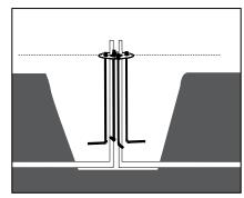
Run conduit inside of the anchor plate center hole prior to pouring concrete. The conduit may project above the finished surface of the concrete by 3/8" maximum.
