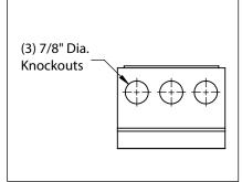
Stainless steel housing has three (3) 7/8" diameter knockouts located on bottom of housing.
