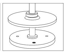
Attach mounting plate to suitable enclosure in final fixture location according to designed lighting plan using appropriate hardware (By Others). Seal as per NEC.
