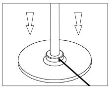
Slide canopy cover and locking ring over mounting plate and tighten set screw using a 5/64" Allen wrench.
