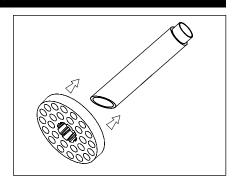
Slide Stability Flange onto Power Pipe II<sup>™</sup>. Use Stability Flange to aid in installation of Power Pipe II<sup>™</sup>.
