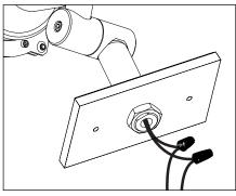
1. Mount fixture onto suitable enclosure according to designed lighting plan. Use locknut to secure.
