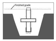
Pull secondary wiring from remote driver to Power Pipe™. Allow for additional cable to make connections to fixture lead, future service and stem length adjustment. Place Power Pipe™ in hole
