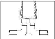
Connect conduit to the conduit couplers attached to the bottom of the Power Pipe™. Place Power Pipe™ in hole.
