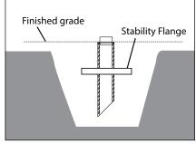
Excavate trench according to designed lighting plan. Dig hole a minimum of 24" deep and 10" wide to accommodate Power Pipe II™ at desired fixture locations.
