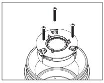
Gently lift LED module and disconnect from fixture. Install new LED module. Secure set screws through LED module and optic holder using .050" Allen wrench.
