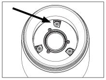
4. Use .050" Allen wrench to loosen three (3) set screws holding optic holder and LED module.
