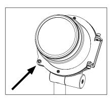
8. Tighten two (2) captive screws on stainless steel clamp rings using 5/32" Allen wrench. Do not overtighten.
