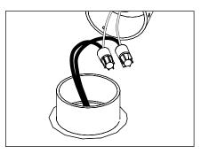
Make waterproof connections from remote driver secondary side to fixture secondary leads using waterproof wire connectors. See wiring diagram.
