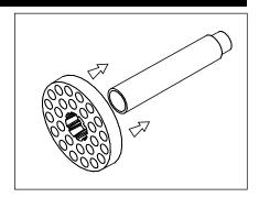
Slide Stability Flange onto Power Pipe™. Use Stability Flange to aid in installation of Power Pipe™.
