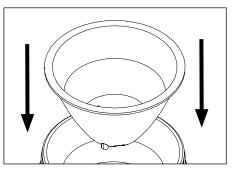
Replace optic by lining tabs with optic holder, then pressing down gently until secured into place.
