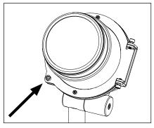
Loosen two (2) captive screws on stainless steel clamp rings using 5/32" Allen wrench until the screws disengage from back plate.
