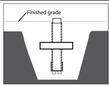
Excavate trench according to designed lighting plan. Dig hole a minimum of 24" deep and 10" wide to accommodate Power Pipe™ at desired fixture locations.
