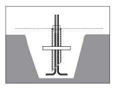
Pull low voltage wiring from remote driver to Power Pipe II™. Allow for additional cable to make connections to fixture leads and future service. Place Power Pipe II™ in hole.
