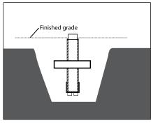
Excavate trench according to designed lighting plan. Dig hole a minimum of 24" deep and 10" wide to accommodate Power Pipe II™ at desired fixture locations.
