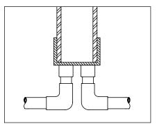
Connect conduit to the 3/4" conduit couplers attached to the bottom of the Power Pipe II™. Place Power Pipe II™ in hole.
