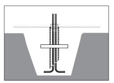
Pull low voltage wiring from remote driver to Power Pipe II™. Allow for additional cable to make connections to fixture leads and future service. Place Power Pipe II™ in hole.
