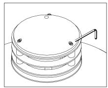
Place cap back on fixture body. Tighten three
