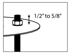
Adjusted anchor bolts to project at least 1/2" but no more than 5/8" above the anchor plate after installation. The four (4) 1/4-20 nuts on top of the plate may be left in place while concrete is
