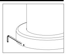
Slide decorative base over mounting tenon and base, then secure with three (3) #8-32 set screws using 5/64" Allen wrench.
