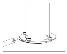
Seal as per NEC with waterproof silicone sealant (By Others).
