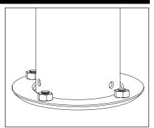
Secure to anchor bolts with the 1/4-20 nuts and lockwashers provided with the #34 Anchor kit using adjustable crescent wrench.
