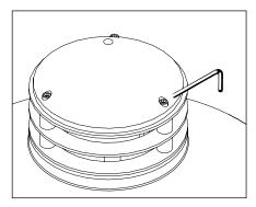
1. Loosen three (3) #8-32 set screws on cap using 9/64" Allen wrench.
