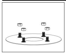
Remove 1/4-20 nuts from installed #34 anchor kit with adjustable crescent wrench.
