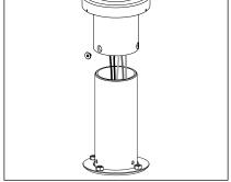
Place wiring connections inside of tenon. Secure fixture body to tenon with three (3) 1/4-20 set screws u sing 3/16" Allen wrench.
