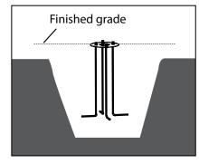
Install anchor plate and bolt assembly flush with the finished grade.
