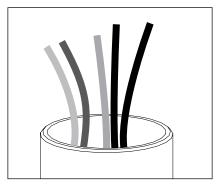
Pull primary branch circuit wiring and any additional dimming controls or other wiring necessary for installation (By Others.)
