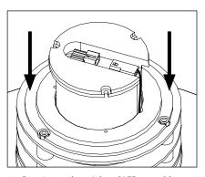
4. Drop in new heatsink and LED assembly.
