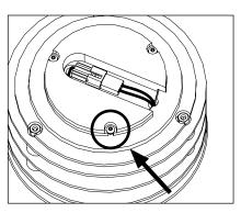
6. Tighten three (3) screws at top of heatsink using 3/32" Allen wrench.
