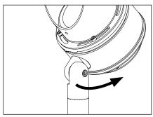
Use 5/32" Allen wrench to loosen #10-32 stainless steel black oxide socket head cap screw at the knuckle for vertical aiming purpose.
