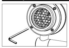
Use 9/64" Allen wrench to loosen (4) #8-32 stainless steel socket head screws to remove lens
