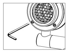
7. Re-install lens bezel. Tighten evenly.
