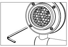
Use 9/64" Allen wrench to loosen (4) #8-32 stainless steel socket head screws to remove lens bezel.
