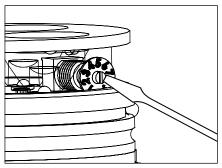
With small flat head screw driver rotate Adjust-e-Lume® dial to desired lumen output.
