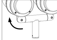
Use 5/32" Allen wrench to loosen #10-32 stainless steel black oxide socket head cap screw at the knuckle for vertical aiming purpose.
