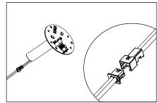
Disengage LED board and driver assembly. Replace with new board and driver assembly.
