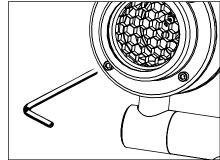
7. Re-install lens bezel. Tighten evenly.
