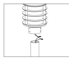
Make watertight connections using waterproof wire connectors to connect fixture leads to secondary leads from driver. Leave length for future service. See wiring diagram.
