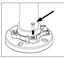
Close hinge pole, then secure to base with three (3) 1/2" I.D. flat washers, split lock washers and three (3) 1/2"-13 stainless steel bolts using an adjustable crescent wrench.
