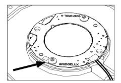
Loosen two (2) #4-40 button head screws with 4. 1/16" Allen wrench.
