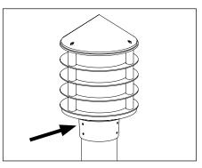
Secure with six (6) 1/4-20 socket head set screws using 1/8" Allen wrench. Make sure the fixture is completely seated. Do not overtighten.
