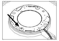
7. Spread thin, even layer of thermal paste on back of new LED module.
