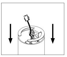
3. Place connections and driver on bracket into pole. Rest bracket on pole top or tenon.
