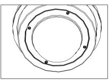
3. Loosen four (4) #4-40 socket head set screws on side of dome lens optic holder using 3/32" Allen wrench. Gently remove dome lens.
