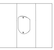
7. Close hand hole cover with hardware and tools as per pole manufacturer. (Pole and Hardware By Others)
