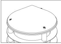
Loosen three (3) captive #10-24 socket head screws on cap with 5/32" Allen wrench. 1.
