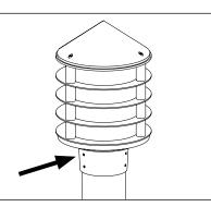
Slide fixture over pole top. Secure with six (6) 1/4-20 socket head set screws using 1/8" Allen wrench. Make sure the fixture is completely seated. Do not overtighten.
