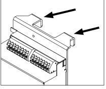
Driver bracket should hang off small horizontal interior bar inside pole near hand hole. Use two hooks on bracket to hang on interior bar.
