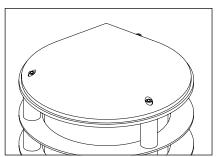
11. Attach cap with securing three (3) #10-24 socket head screws using 5/32" Allen wrench.
