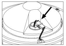
2 Disconnect quick disconnects at top of heatsink.
