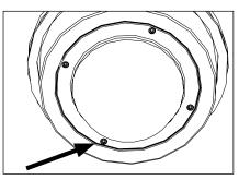
9. Place dome lens onto heatsink. Tighten four (4) #4-40 socket head set screws on side of dome lens optic holder using 3/32" Allen wrench.
