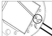
6. Use small pick tool to push connector off LED board through two small slots behind connector. Once loose, lift connector upwards and off board.
