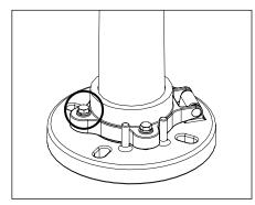
1. Remove base cover (if required). Open hinge base on pole by loosening three (3) 1/2"-13 stainless steel bolts using adjustable crescent wrench.
