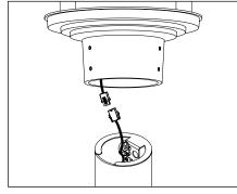
Make secondary connections via quick disconnect from driver secondary side to fixture secondary side.
