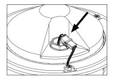
10. Attach heatsink to fixture body via quick disconnect. Line up on spacers.
