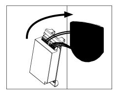
5. Place connections and driver on bracket into pole through hand hole. (For use with 3"x5" hand hole).
