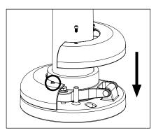
If pole comes with cover, place cover on base of pole. Secure with four (4) 1/4"-20 hex screws using 3/16" Allen wrench.
