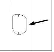
Open hand hole as per pole manufacturer's instructions, then pull primary branch circuit wiring through conduit to splice location and 3. pull down fixture leads from installed pole top.
