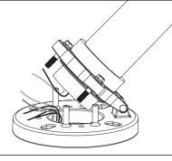
2. Hinge pole open for access to conduit and branch circuit wiring. Pull branch circuit wiring and dimming controls to splice location.
