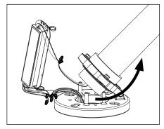
4. Place driver, bracket and connections into pole. Hinge pole back to upright position. Connect secondary wiring to secondary side of driver. Pull secondary wiring to top of pole. Length of secondary wiring will vary with height of pole. Leave length for future service.
