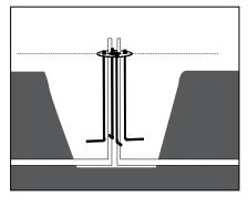
Run conduit inside of the anchor plate center hole prior to pouring concrete. The conduit may project above the finished surface of the concrete by 3/8" maximum.
