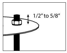
Adjusted anchor bolts to project at least 1/2" but no more than 5/8" above the anchor plate after installation. The four (4) 1/4-20 nuts on top of the plate may be left in place while concrete is poured.
