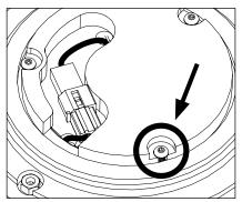
Tighten three (3) screws at top of heatsink using 3/32" Allen wrench.
