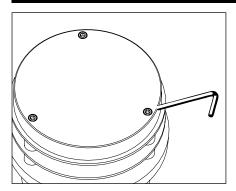
Loosen three (3) #8-32 set screws on cap using 9/64" Allen wrench.
