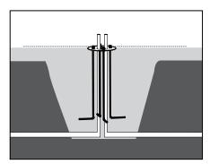
With the conduits in place and the anchor plate properly positioned, secured and leveled, concrete may be poured.
